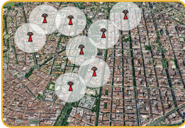
FIG 1 Example of 8 RSUs deployed following the minimum cost deployment policy.
