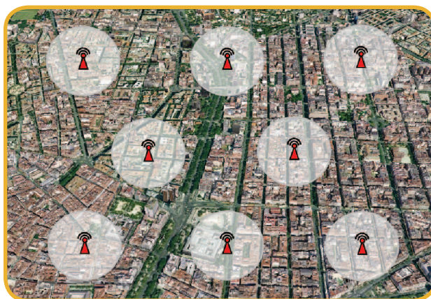
FIG 2 Example of 8 RSUs deployed following the uniform mesh deployment policy.
